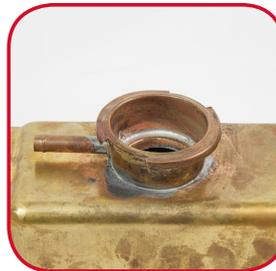
The filler neck is reinforced with internal and external brazing.
